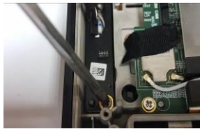
Loos screws of 2M CAM modules
