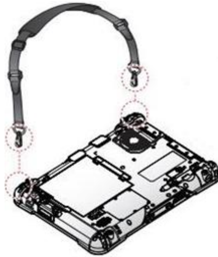
Figure 37. Removing the Shoulder Strap
