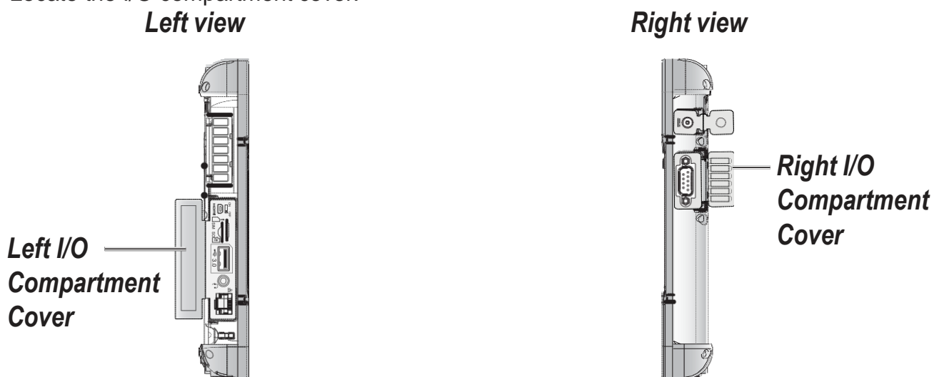
Figure 20. Side View: Locating the I/O Compartment Cover
