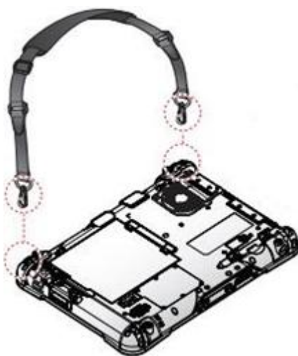
Figure 36. Connecting the Shoulder Strap
