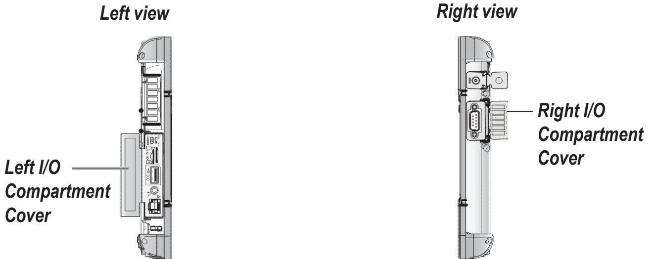
Figure 17. Side View: Locating the I/O Compartment Cover
