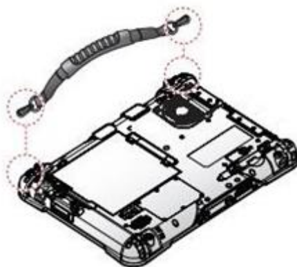
Figure 34. Connecting the Handle
