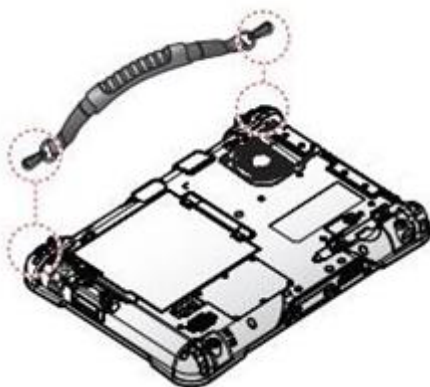
Figure 35. Removing the Handle
