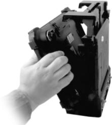
3. Push tablet forwards and make sure tablet is well connected and fixed with latches.
