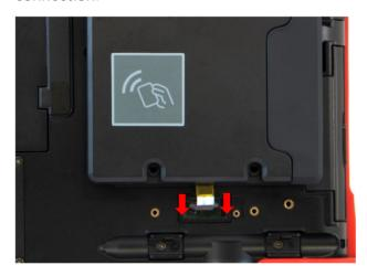
I-6. Align the SnapON module to the four screw holes and secure it with provided screws.
