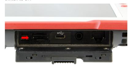
I-2. Place the device display side down on a clean work surface and release the screw of expansion by cover.
