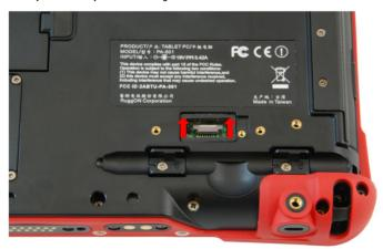
I-4. Connect the FFC cable (pin face up) to the connector.
