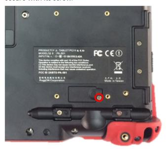
II-6. Install the battery and set the DIP switch to ON.
