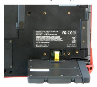
I-5. Make sure the cable is fully connected and push the connector clip to secure connection.
