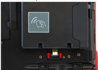
II-4. Remove SnapON module. Keep the SnapON module and its screws for future use.
