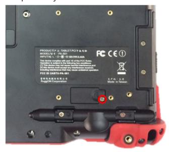
I-3. Remove expansion bay cover and pull the expansion connector clip to unlock. Keep the expansion by cover and its screw for future use.
