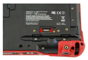
II-5. Push connector clip to its original place. Align the expansion bay cover and secure with its screw.
