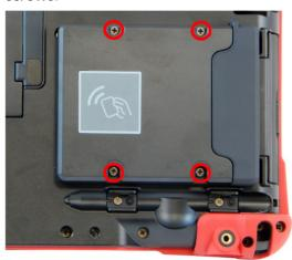
I-7. Install the battery and set the DIP switch to ON.
