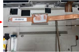
Tear off the Metal sheets
