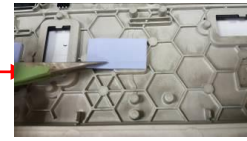
Take off Tear off Thermal Pad
