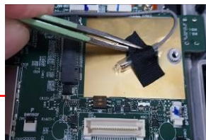
Take off the GPS antenna cable
