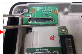
Take off the PCBA USBC Docking Board(S.S.T.)
